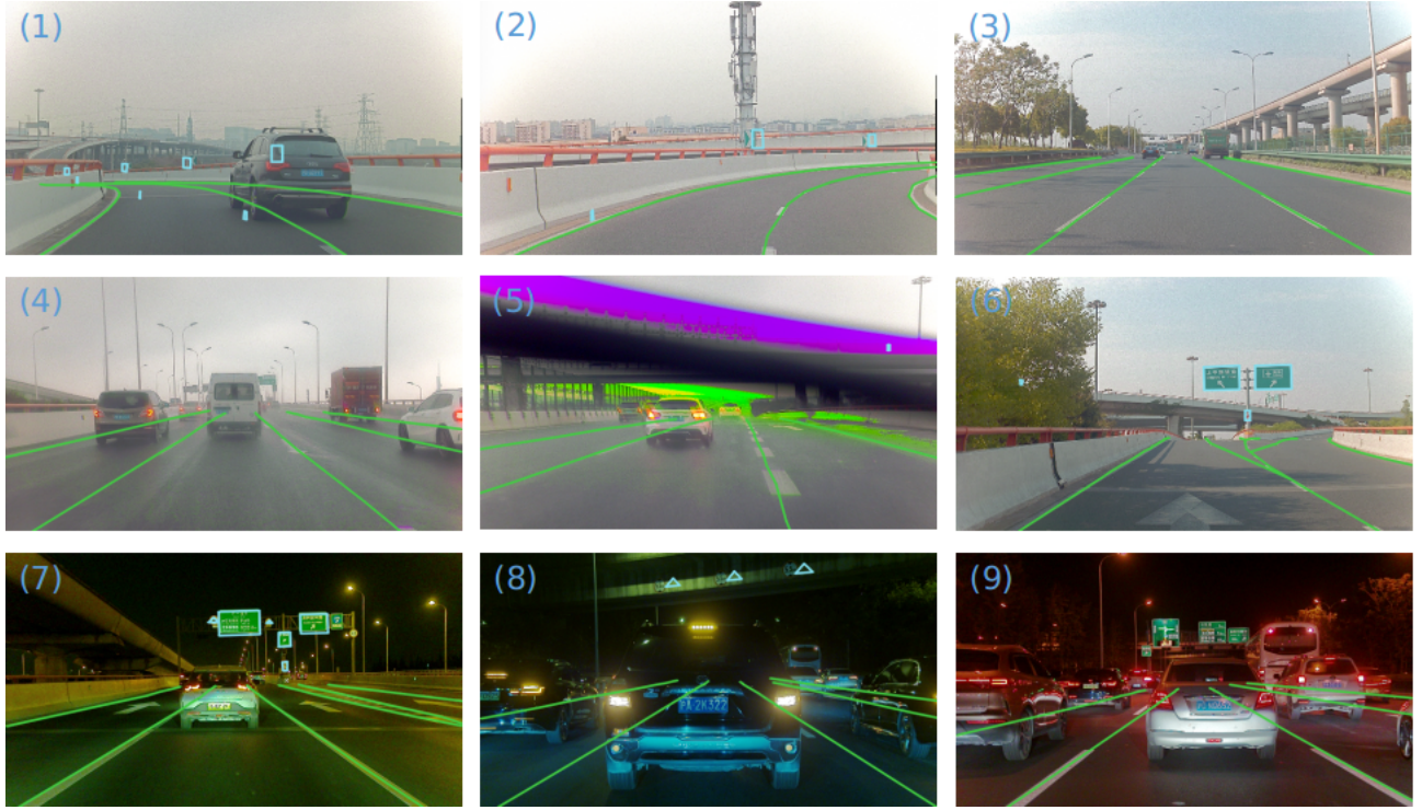
Fig. 6. Qualitative results on Shanghai dataset. Projection results of different scenes: (1-2) curve road; (3) long straight road in sunny day; (4) rainy; (5) windshield wiper blocks part of the image; (6) diverging ramp; (7) low illumination; (8-9) traffic jam.
